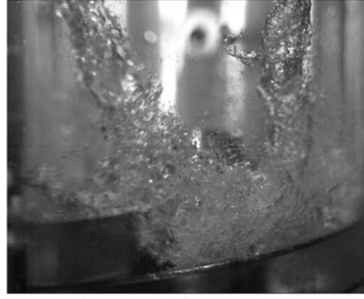
b) Water at 337 K: \omega_{inducer} = 5973 rpm, \sigma = 0.058 , \phi/\phi_{max} = 0.45 , \psi/\psi_{max} = 0.55 , \omega/\omega_{inducer} = 0.29 , d/d_{inducer} = 0.69 , \delta/d_{inducer} = 0.10
