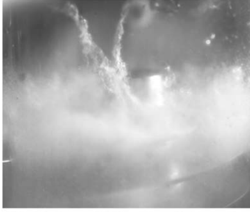
a) Liquid nitrogen at 77.5 K: \omega_{inducer} = 4448 rpm, \sigma = 0.059 , \phi/\phi_{max} = 0.47 , \psi/\psi_{max} = 0.53 , \omega/\omega_{inducer} = 0.28 , d/d_{inducer} = 0.72 , \delta/d_{inducer} = 0.046
